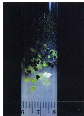
Fig. 15. Gel growth of silver periodate by pH reduction ( AgNO_3 , H_2IO_6 , and sodium silicate gel). Yellow crystals: Ag_2H_3IO_6 , red-brown crystals (black in photograph): Ag_2IO_5 [124].
